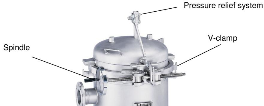
The QIC-LOCK mechanism is a two piece V-shaped clamp that can be opened and closed using a hand operated spindle mechanism. The V-shape closes over the housing and cover flange that seals with an O-ring. The V-clamp is then locked by closing a handle that closes a pressure relief device. This device needs to be opened first in order to operate the spindle.
