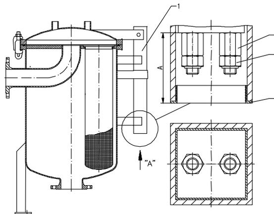
For re-adjustment the dust cap below the spring lift device is to be removed. When viewed from below two threaded bars with hex-nuts can be seen. Two hex-nuts are secured with additional self-securing hex-nuts to guard against misalignment and removal through counters. The counter hex-nuts must be loosened.
