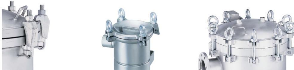
To open the housing first loosen the eye nuts on the top. The eye nuts can be loosened using a small bar. Where hexagon nuts are used the appropriate wrench should be used. If swing bolts are used the nuts should be loosened enough to allow for them to be swung clear of the cover. Similar procedures are to be followed for segment clamp-screws. If stud bolts are used the nuts must be removed completely.
