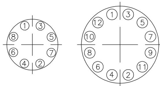
When using maximum allowable torque the bolts are to be tightened in three steps.
