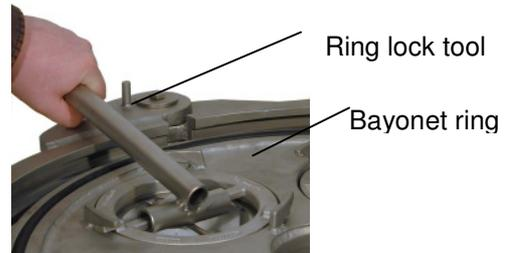
Bag-fixing rings for FLOWLINE and SIDELINE housings have a spring steel band for hold down. The pressure is provided by the cover of the filter housing. It is important that the pressure is applied onto the sealing ring of the filter bag. If it does not the bag-fixing ring may need to be adjusted.
