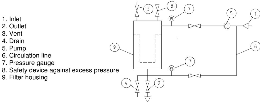
The filter housing in the example given is equipped with shut-off devices for discharge and venting. Pressure gauges for measuring the differential pressure are installed in the inlet and outlet connections.
