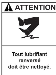
LE LUBRIFIANT DE LA POMPE EST TRES GLISSANT, ET PEUT OCCASIONNER DES BLESSURES GRAVES. IL EST IMPERATIF D'EN NETTOYER TOUT ECOULEMENT.
