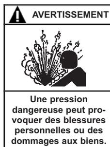
LA PRESSION HYDRAULIQUE DOIT IMPERATIVEMENT ETRE COMPLETEMENT RELACHEE AVANT CHAQUE OPERATION DE MAINTENANCE AFIN D'EVITER DES DOMMAGES CORPORELS OU MATERIELS.
