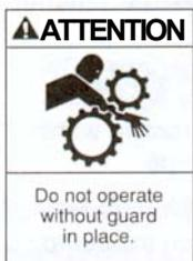
**AVANT DEMARRAGE, S'ASSURER QUE LES PROTECTIONS (COUVERCLE, FENETRE, CAPOT DE VENTILATEUR, CARTER D'ACCOUPEMENT, ETC.) SONT EN PLACE ET FIXES.**
